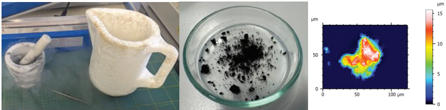
Figure 3: from left to right: LN2 milling of pad material; grinded pad material particles; confocal microscopy image of pad material particle
