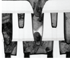
Figure 1. TEM image of the fill defect in a copper via. Image taken after anneal and CMP.
